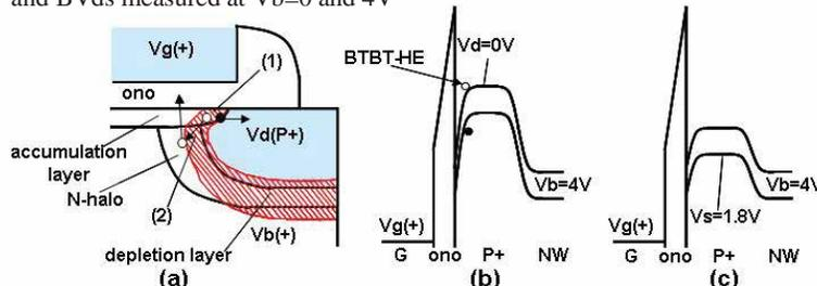
Fig.3 (a) Back bias assisted BTBT-HE generation consists of 2 steps, (1) BTBT generation, (2) electron acceleration, (b) band diagram at drain edge, BTBT-HE is generated, and (c) band diagram at source edge, BTBT is inhibited by  $V_s=1.8V$
