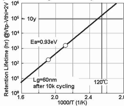
Fig.10 Retention lifetime estimation
