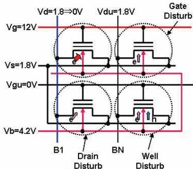
Fig.4 Programming and disturb conditions in NOR array
