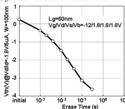
Fig.8 FN hole injection erase characteristics
