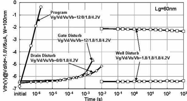
Fig.5 Programming, drain, gate and well disturb characteristics
