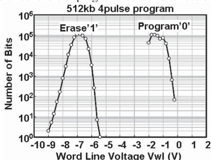
Fig. 5 Threshold voltage distributions for SLC operation.
