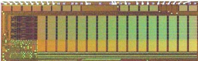
Fig. 1 Die photograph of 4Mb B4-Flash test chip.
