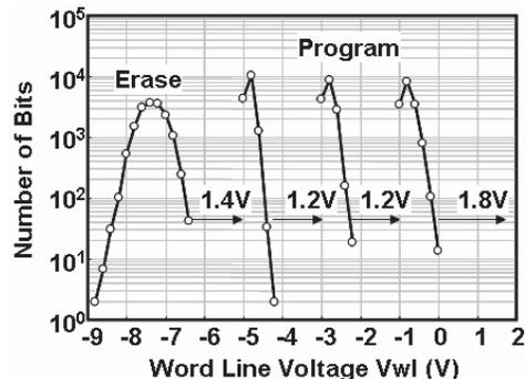
Fig. 6 Threshold voltage distributions for MLC operation.
