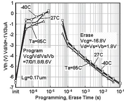
Fig.7 Temperature dependence of program and erase characteristics
