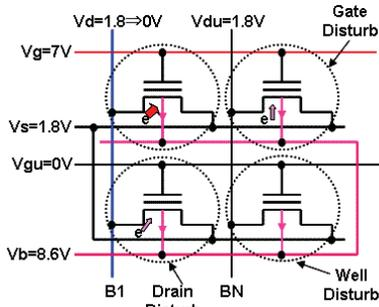
Fig.5 Program and disturb conditions in NOR array
