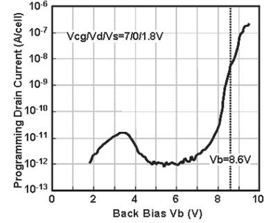
Fig.8 One-shot programming drain current
