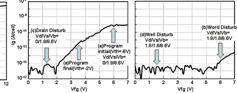
Fig.4 Gate current comparison, (a)program selected, (b)word-disturbed, (c)drain disturbed and (d)well-disturbed cells
