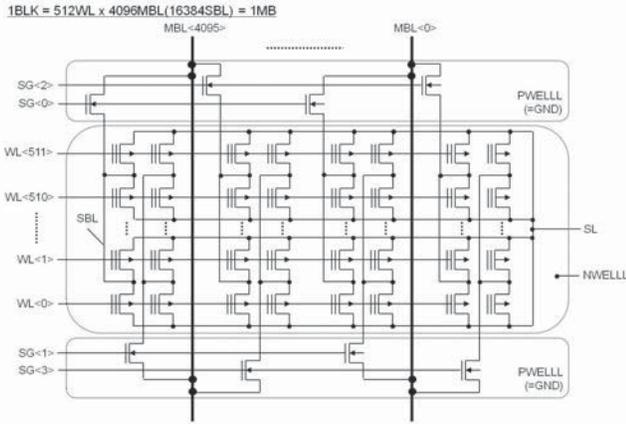
Figure 2. Memory cell array architecture
