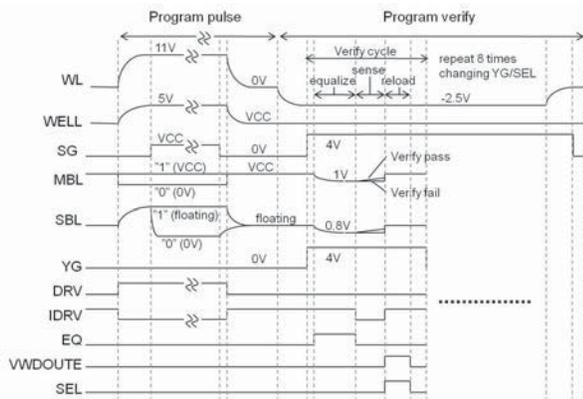
Figure 4. Timing diagram of program operation
