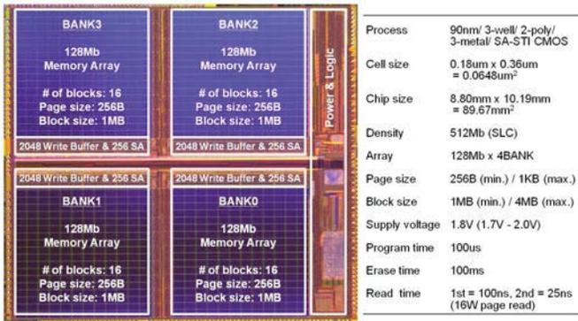
Figure 1. Die microphotograph of 512Mb B4-Flash memory
