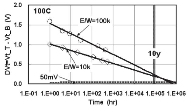
Fig.9 Comparison of 100C retention characteristics of the 100k cycled element with that of 10k cycled element.
