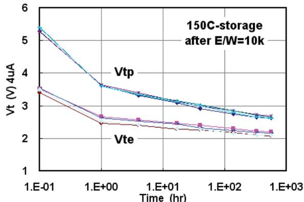
Fig. 6 Typical data retention characteristics at 150C after 10k cycling, using 10 elements.
