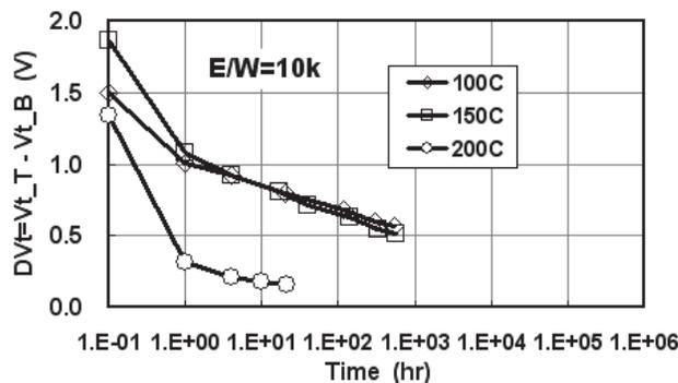
Fig.7(a) Temperature dependence of data retention characteristics after 10k cycling.
