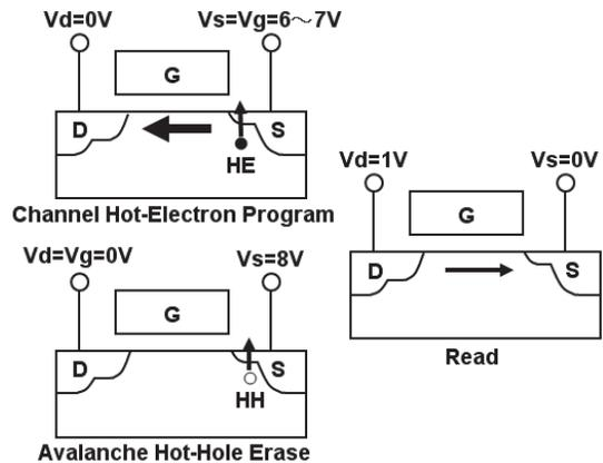
Fig.2 eCFlash element structure and its operation.
